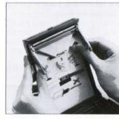
B. ローラーをはずすには、両側の U字形金具を両手でいっしょに持ち 上げると、はずれます。 B. Lift up the U-shaped metal on both sides at the same time, which will permit the roller assembly to be detached. Detach the assembly and check the rollers carefully.
